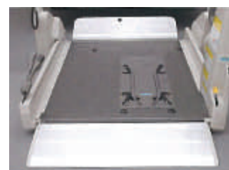
Built-in lift with wheelchair support hooks for safer access. ↓
